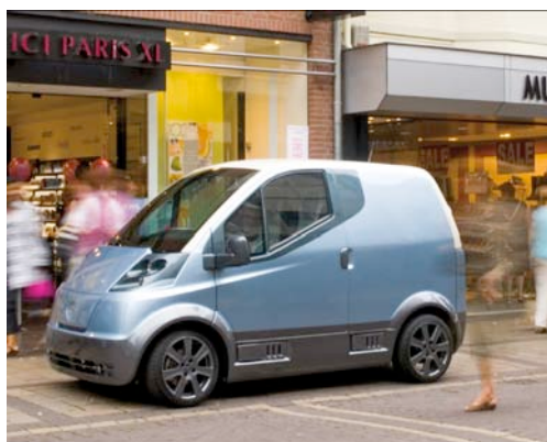
QUICC! DiVa (DistributionVan) - electrically powered lightweight plastic car by DuraCar ( www.quicc.eu )
