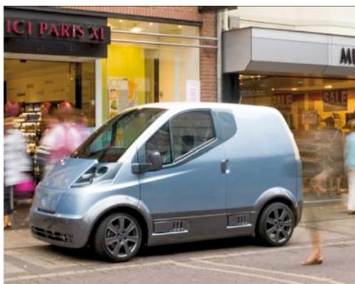
QUICC! DiVa (DistributionVan) - electrically powered lightweight plastic car by DuraCar ([www.quicc.eu](http://www.quicc.eu))
